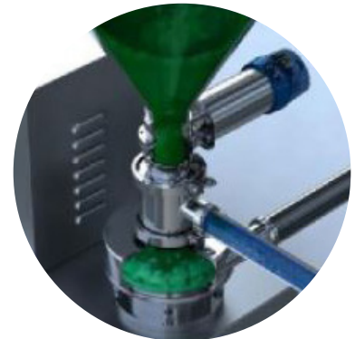
The mixture is transported to the tank equipment
