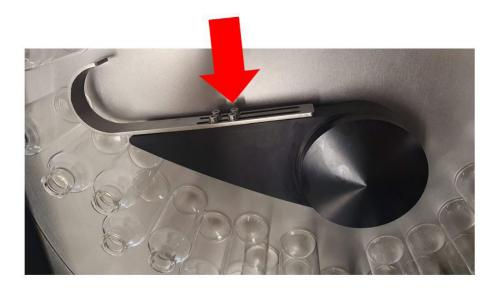
3. Adjust the dispensing needle to the centre of the bottle. The needle holder has two handles to adjust the needle vertically (according to vial height), as well as the angle and depth with respect to the centre of the holder (according to vial diameter).
