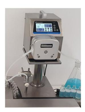
There is a third handle to change the dispensing needle due to maintenance or because the process requires a different size.
